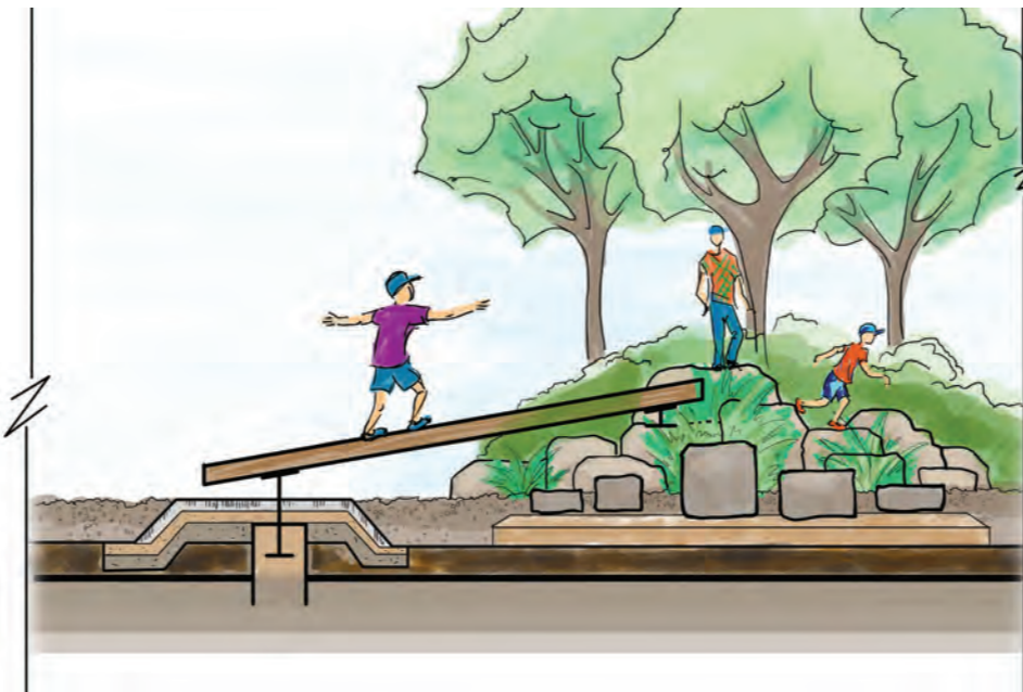
2 Log hop to rock drop - Typical section Scale 1:50 @A3
