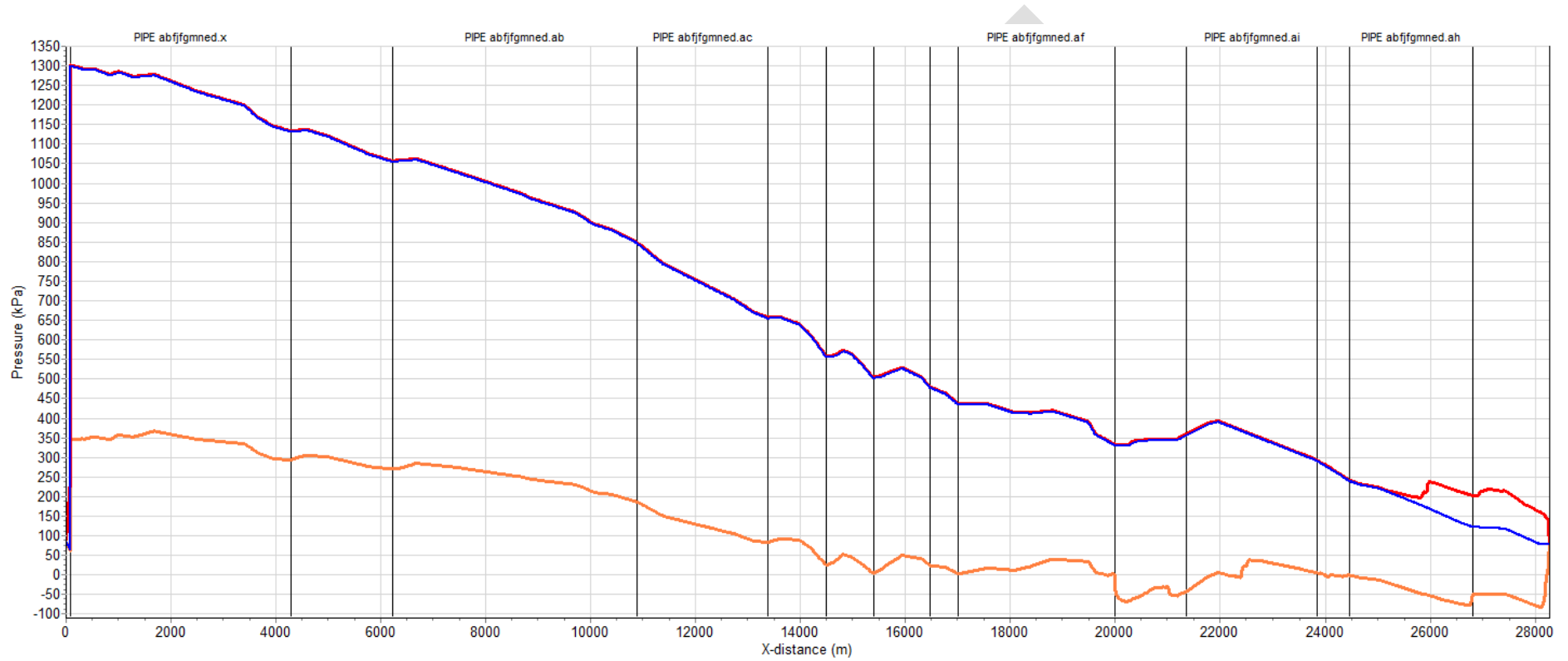
Figure 5.22 NERPS protected pressure envelope
