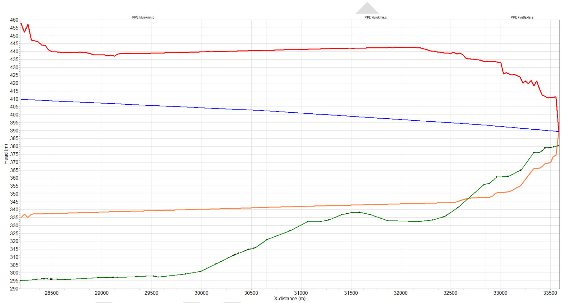
Figure 5.23 ARPS unprotected hydraulic envelope
