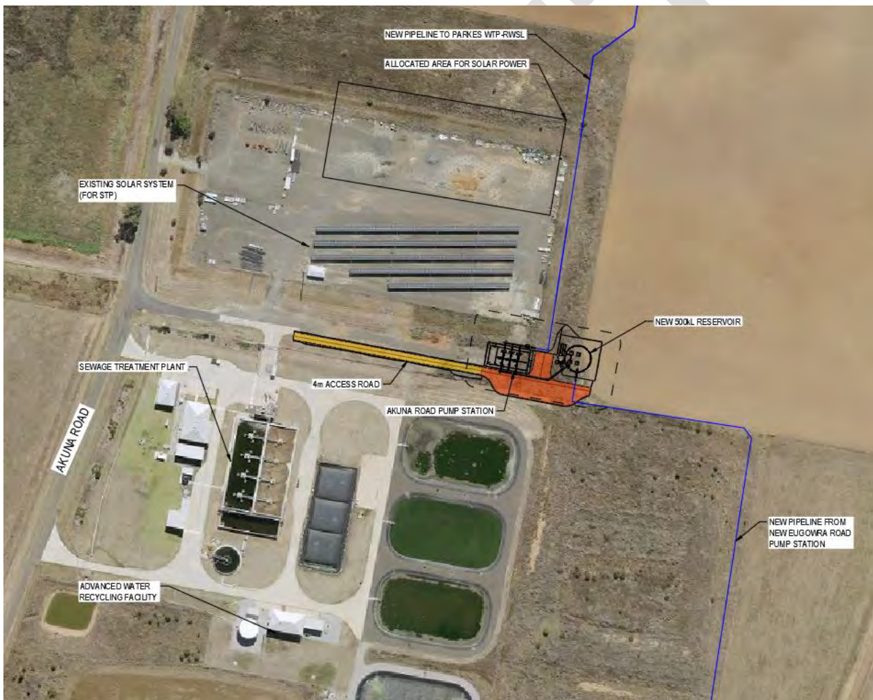
Figure 7.1 Akuna Road Pump Station Layout
