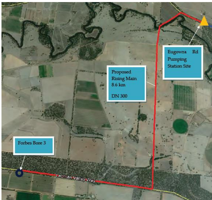
Figure 3.5 Centroc Water Grid Connection to Forbes Bore 3
