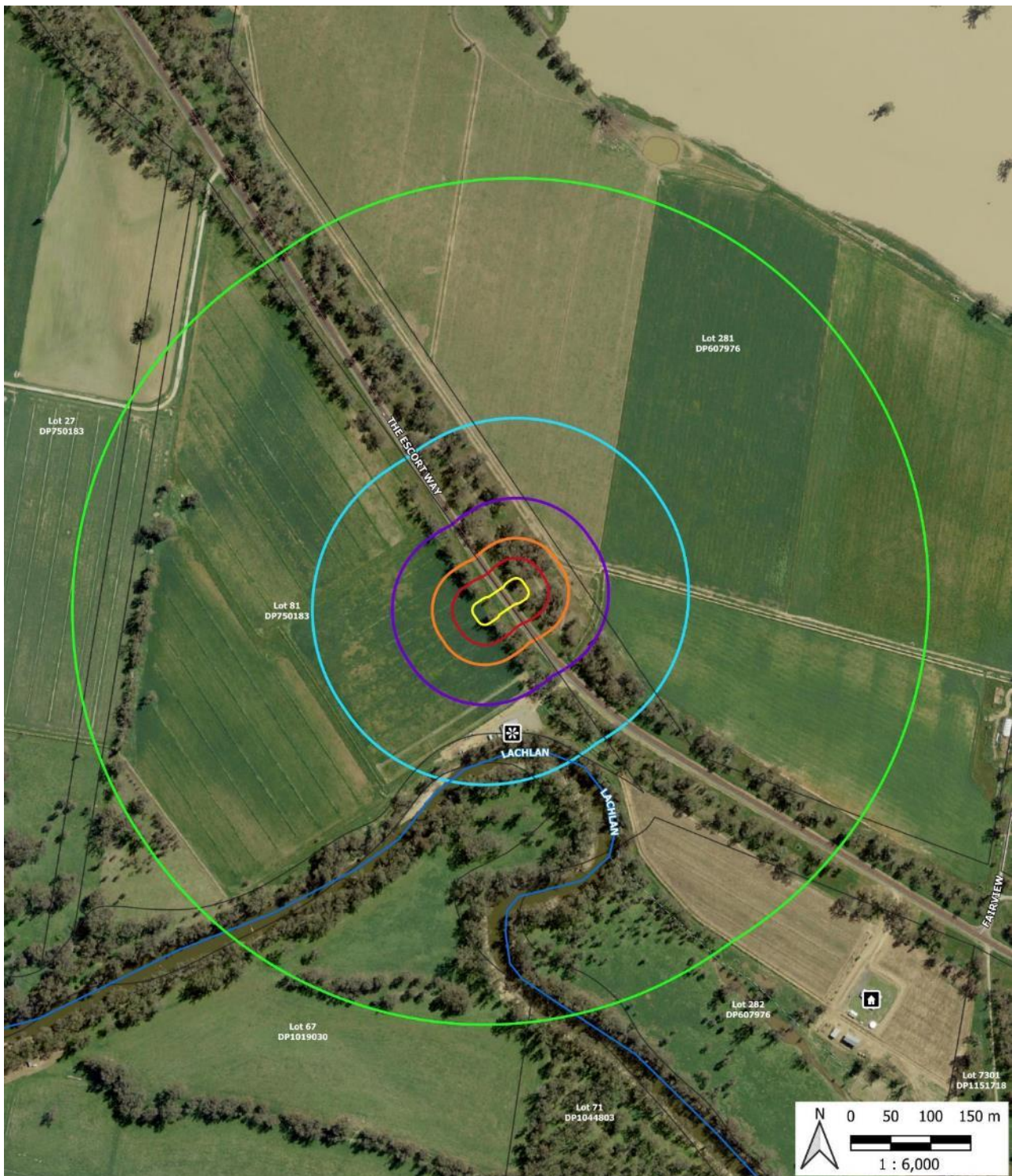
PSC The Escort Way Underbore - Sensitive Receivers within a 500 m radius of Proposal location
