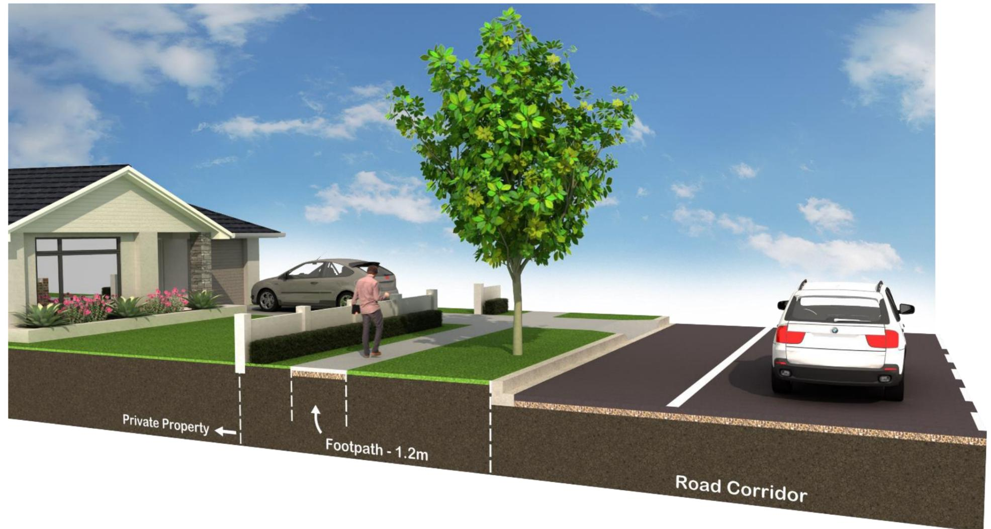
Concept Drawing - Typical 1.2m wide footpath installation on a road with kerb and gutter
