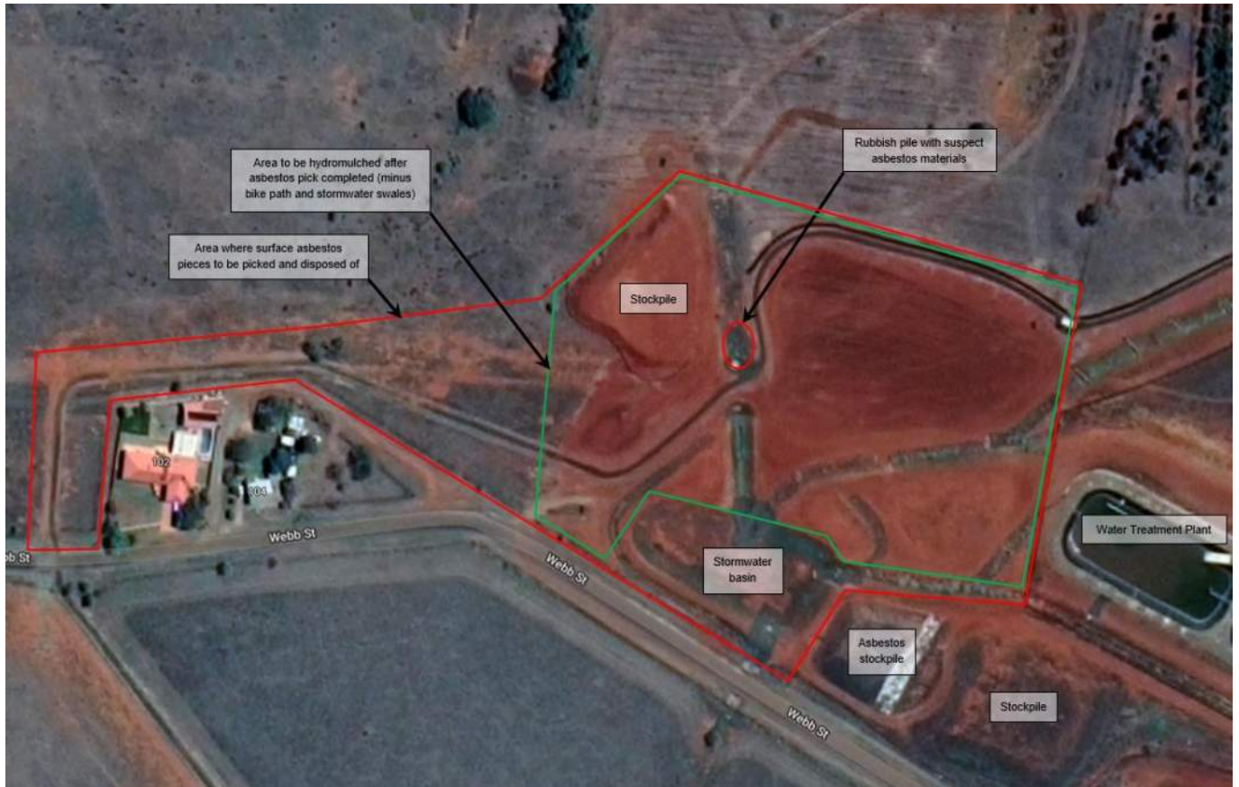
Figure 3: WTP Asbestos Sketch
