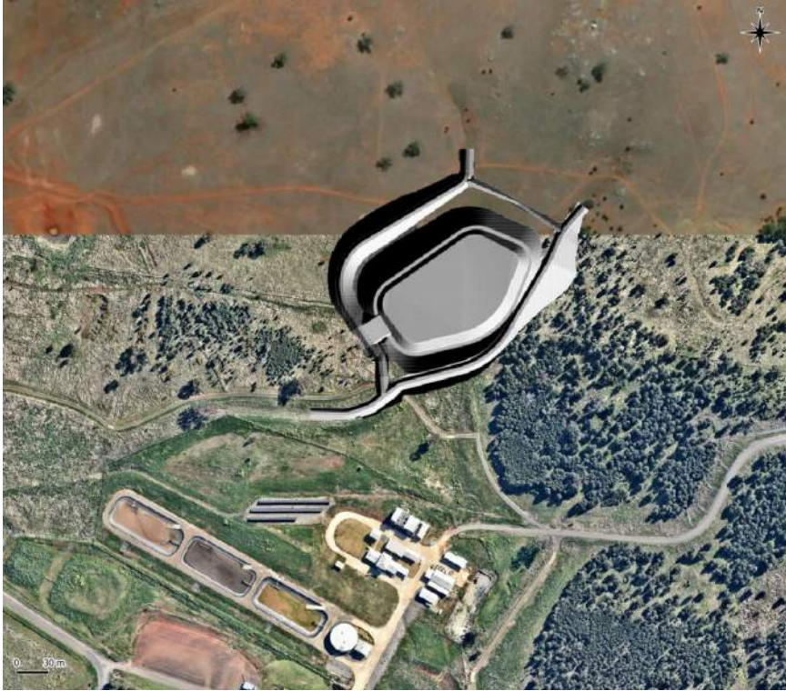
Figure 2: WTP Raw Water Storage Lagoon Layout
